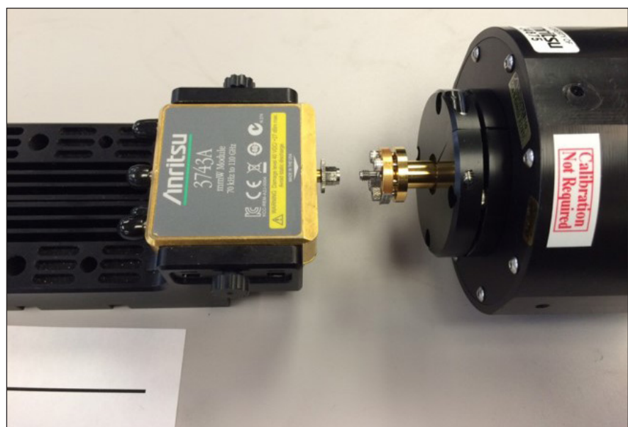
Figure 18: Anritsu VectorStar VNA 110 GHz based setup and its components for free space material measurements
